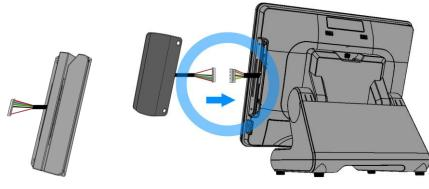
3. Tighten the two PHILLIPS M3 screws to fix the MSR assembly as shown below.
