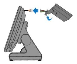
3. Mount the customer display to the device and tighten the two PHILLIPS M3 screws as shown below.
