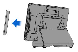
2. Connect the cable of the MSR assembly to the device.
